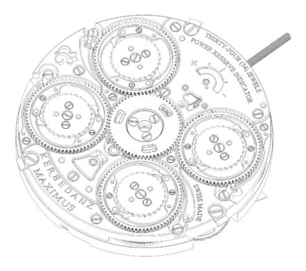
and its power reserve, which is displayed in a separate indicator, offers a remarkable autonomy of 54 hours. The watch has a total of 415 components, 73 of which belong to the tourbillon cage made of titanium and weighing 1.35 grams. It should be noted that titanium is lighter than steel, that it resists well to magnetic aggressions and that the cage revolves in 6 minutes instead of the usual 60 seconds.
